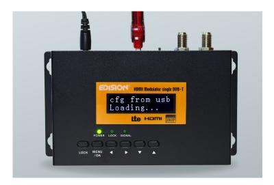
HDMI MODULATOR re-boot with the new config file, as set by the user
